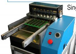
Singulate multiple prescored PCB panels in one pass with the FKN Systek K5000 or K6000 PCB depanelizer. Panels up to 10" wide can be separated by placement onto an input conveyor to be passed onto the separator blades.
