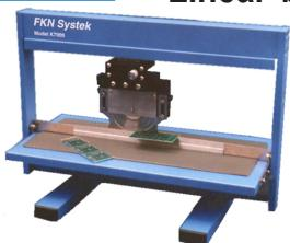
The K7000 is a circular on linear blade depanelizer developed to singulate prescored PCBs with very tight component spacing. The linear blade is 12" (304mm) long and has a .030" (.762mm) thin symmetrical cutting edge designed particularly for PCBs with closely spaced components. The circular blade is 3.8" (96.52 mm) in diameter and has the same cutting edge profile as the linear blade.
