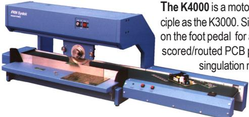
The K4000 is a motorized linear blade depanelizer working on the same principle as the K3000. Simply place the PCB scoreline on the linear blade and step on the foot pedal for automated singulation of prescored panels. Scored and scored/routed PCB panels are safely separated by the linear circular blade singulation method. Blades are made of long lasting tool steel and are slightly rounded. Available in standard 18" linear blade or long 24" linear blade versions.
