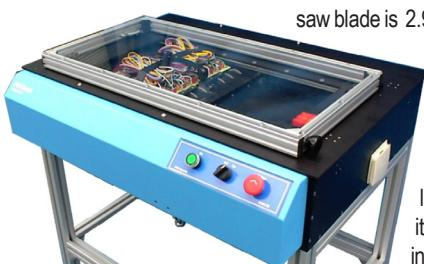
The S series diamond blade depaneling saws are used to singulate assembled PCBs. The saw blade is 2.95" (75mm) diameter .021" thick. On the S100 an adjustable front and back blade guard assure that the PCB is held at the correct height to cut just deep enough for clean board singulation.
