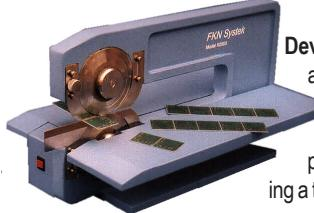
Developed for low cost singulation of panelized printed circuit cards, the K1000 and K2000 are a hand operated and motorized version of double circular blade PCB depanelizers which separate panels up to 12.5" in length. The blades are made of long lasting tool steel and can be adjusted for exact positioning for the separation of panels. Blades are easily replaced by removing a threaded holding disk from the main shaft.
