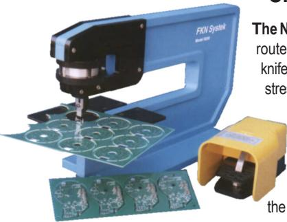
The N200 is a low cost top down air operated punch for singulating tab routed PCB panels one tab at a time. An upper and lower matching knife blade is used to pinch the tabs apart. This method produces less stress on the PCB than a punch and die since the cutting action takes place from both sides.
