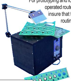
For prototyping and low volume production, FKN has developed the R100 hand operated router system. Dual positioning pins on each side of the router bit insure that the bit can only be inserted in the routed channel to finish routing the tabs.
