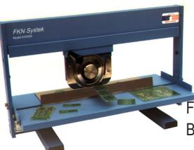
The K3000 manual linear blade depanelizer is designed for singulating longer boards and scored PCBs with skip routed sections. Simply place the scored section on the linear blade and pull the circular blade carriage across the top of the scoreline to split the panels.
